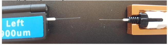
Insert into the splicer like this. And splice.
