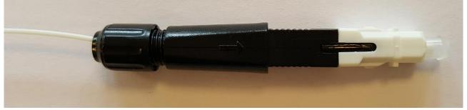
Push the outer housing in place and carefully tighten the relief to the left in picture.
